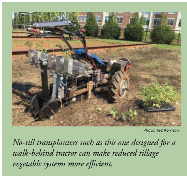
*No-till transplanters such as this one designed for a walk-behind tractor can make reduced tillage vegetable systems more efficient.*
