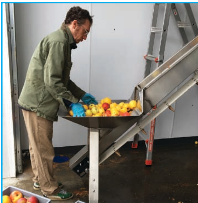
Feeding apples onto an elevator that conveys them to an apple grinder and press
