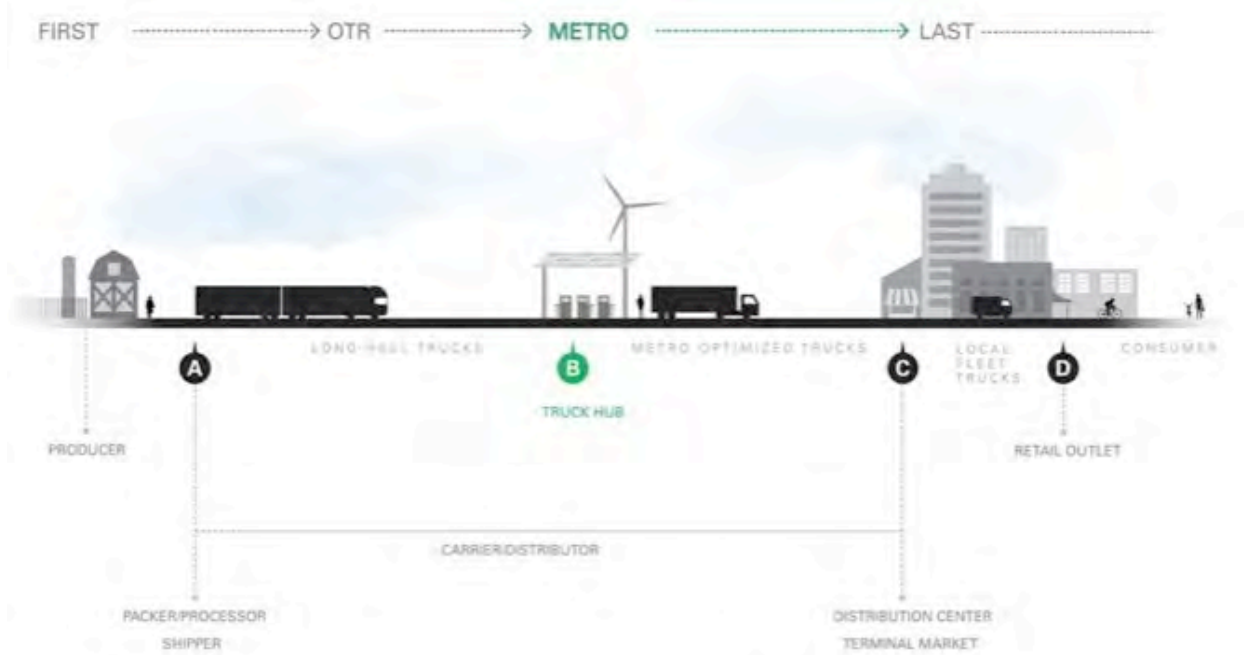
Figure 16. Freight infrastructure innovation: adding a truck hub or drop yard to accommodate "green" shipping into metro regions. Image by Julia Schilling.
